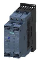
SIRIUS soft starter S2 63 A, 30 kW/400 V, 40  $^{\circ}\text{C}$  200-480 V AC, 24 V AC/DC spring-type terminals Thermistor motor protection
